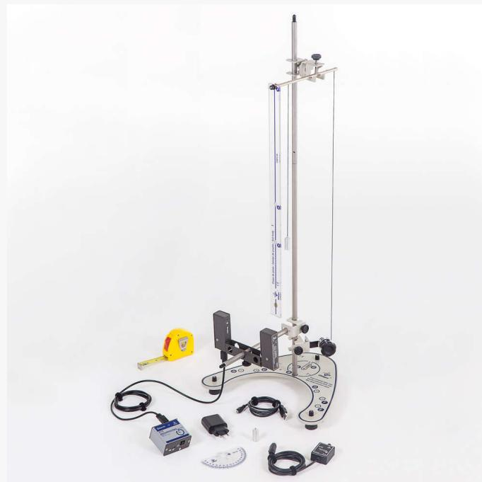
Simple pendulum set and physical bar pendulum, with multichronometer (Bluetooth)
