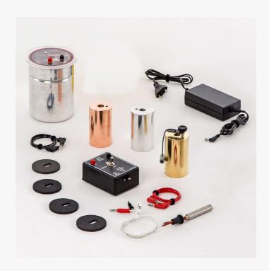
Thermodynamics set, calorimetry, basic, dry, with fixed source, for multimeter with temperature gauge
