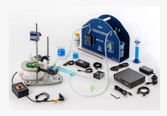
Distillation set with electronic circulating hydraulic flow controller, sensor and interface
