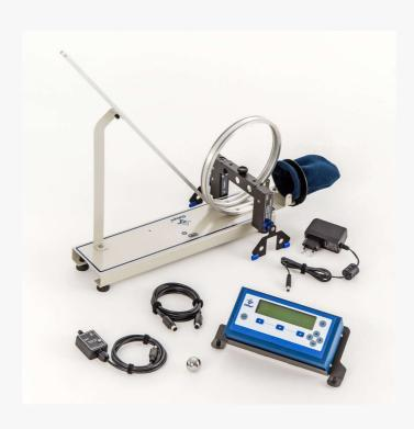
Basic looping with trimmer, analog and digital multimeter and photoelectric sensor
