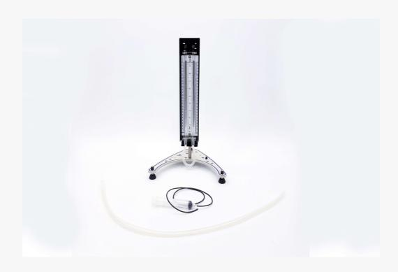
Hydrostatic panel with detachable open tube pressure gauge and tripod
