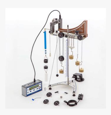
Solid and fluid mechanics set, curved ramp, digital multichronometer 12 functions, sensor
