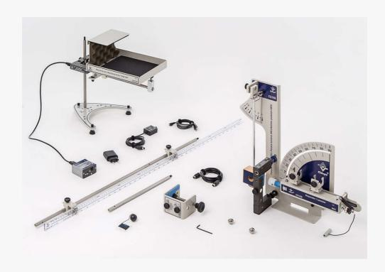
Ballistic pendulum set, bluetooth multi-timer and sensors.
